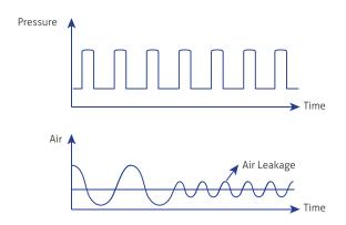
**Smart Detections** If the air leakage reaches 60lpm, it can still be triggered synchronously.
