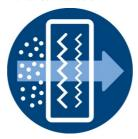
A multi-layer filtration system filters out a wide range of pollutants for superior, long-lasting performance. The pre-filter removes larger dust and hair. Then the true HEPA filter removes ultrafine particles. Finally, an active carbon filter absorbs harmful gases.
